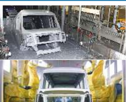
Long Life Rust Protection and Robotic Top Coat for Paint Gloss Retention
